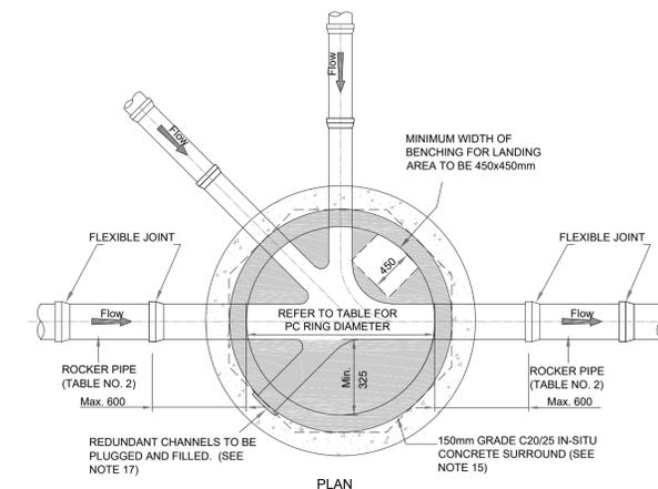
NOTE: IF FLEXIBLE PIPES ARE BEING USED, ROCKER PIPES ARE NOT REQUIRED.
