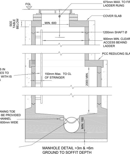
(NOTE: ON MANHOLES <1.5mØ, REDUCING SLAB NOT TO BE USED & PCC RINGS TO CONTINUE UP TO COVER SLAB)
